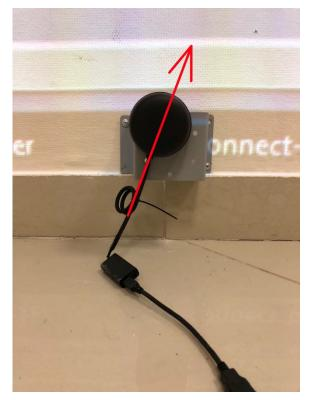
Pic. 20 Determining the direction of the sensor reference axis
