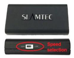
Pic. 4 Selecting the speed of the USB adapter
