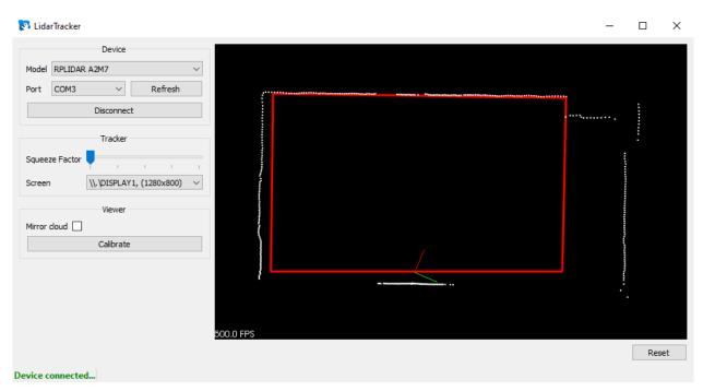
Pic. 32 Set the lower right corner of the projection. Completing the calibration process
